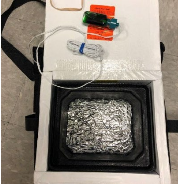
Figure 7: TIC with thermal barrier positioned at base of box
